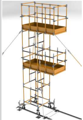
03 Base and Column: 1.0 x 1.0 m Two Platforms: 2.0 x 1.0 m Side Extension: 1.0 m
